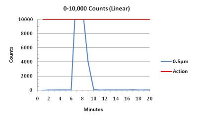
You can see that the graph reaches full scale (10,000 counts/ft³ or 20mA) during the event. The operator or manager when investigating this event has no idea if the counts were just over the action limit or significantly over the limit. In other words it is impossible to determine the severity of the excursion from this graph when using this scale. Clearly the 0-10,000 scale is not suitable. Let us now examine the same data but using the next linear scale available to us.
