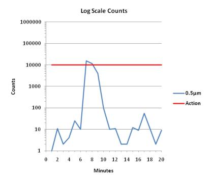
It is now possible to asses the size of the particle excursion and perform an appropriate root cause investigation. It is now possible to distinguish small numbers of particles and very large numbers on the same graph.
