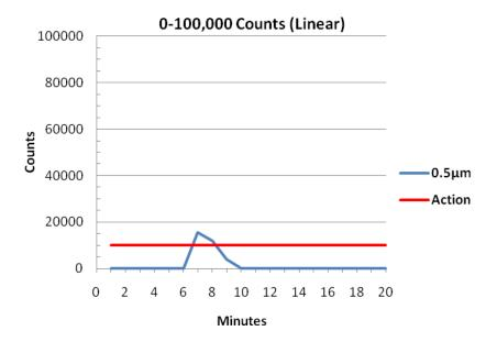
It is now possible to asses the size of the particle excursion and perform an appropriate root cause investigation. It would be possible to measure a very large excursion on this scale. The broad range has now introduced a new problem, it has now become difficult to clearly distinguish low particle counts. Let us now examine the same data but this time using the 4-20 mA Log scaled output.
