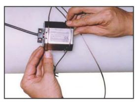
(5) Spread the wire rope near the marked lines in the left-right direction, bring the sensor in close contact and fit the wire rope. Make sure that the matching mark on the sensor is aligned with the marking line.
