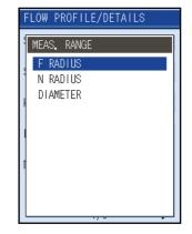
Radius N: Measurement is taken on the radius side adjacent the mounted sensor.
