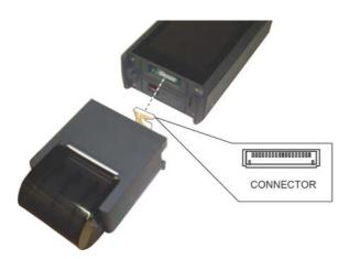
(5) Install the printer with 2 screws.
