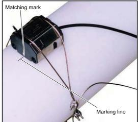
(7) After mounting the upstream sensor, mount the downstream sensor in the same way. The figure is for mounting by the Z method.
