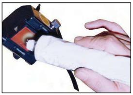
(4) After cleaning the surface of the pipe, the sensor should be mounted.
