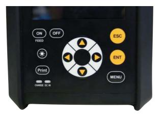
Fig. 4-1 Layout of keys
