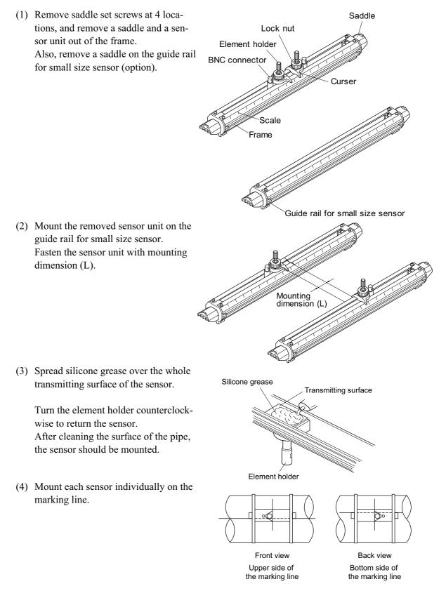
(5) Make sure that the sensor is mounted in parallel with the piping and that the mounting position is correct. Then, turn the element holder clockwise until the sensor is firmly fitted to the piping.
