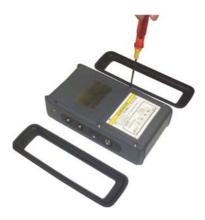
(4) Remove the battery and replace it with the appropriate service part.Note) Install a combination of the main unit side terminal and the battery side terminal.
