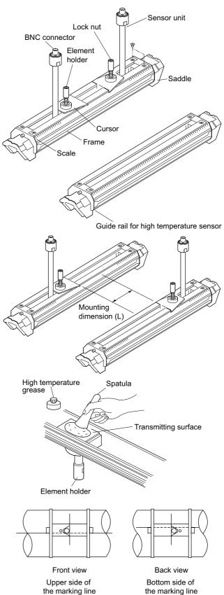
(5) Make sure that the sensor is mounted in parallel with the piping and that the mounting position is correct. Then, turn the element holder clockwise until the sensor is firmly fitted to the piping. Stop turning the element holder where the transmitting surface contacts the surface of pipe, and thus the element holder will not rotate. Do not turn it excessively.
