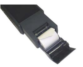
(2) Insert the edge of roll paper into the head assembly.Cut the edge of the recording paper so that central part of it can be inserted first.
