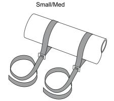
Adjusts the length of the wire rope according to the piping size, fixes the wire on the pipe.
