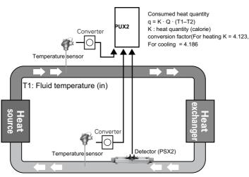
T2: Fluid temperature (out) Q: Flow rate of the fluid
