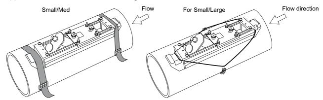
(5) After fastening the sensor to the pipe, screw to the left side, attach the sensor firmly to the pipe.
