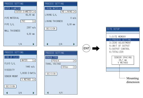
Install the sensor according to chapter 8. MOUNTING OF DETECTOR and the mounting dimension is as displayed on the last line.
