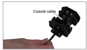
(4) Secure the coaxial cable with the cable clamp.
