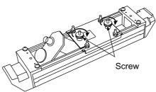
(3) Before mounting the sensor to the pipe, apply grease evenly over the sensor unit and the absorber unit that are to contact the pipe.
