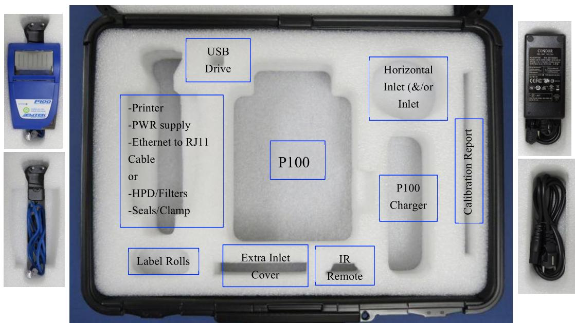
Fig. 1 - P100 Component Placement
