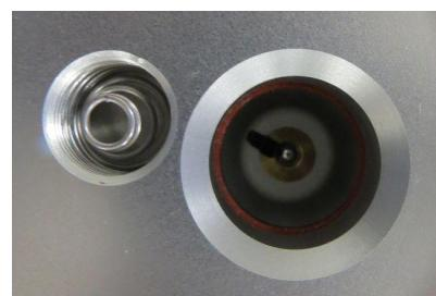
FIG 2 - Stage Tensioning Spring
