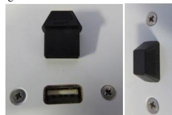
FIG 3- USB Plug Placement
